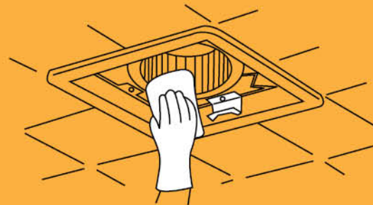
4. Using a cloth dampened with kitchen detergent, remove any dirt from fan body. Wipe dry with new cloth. Replace louver.
