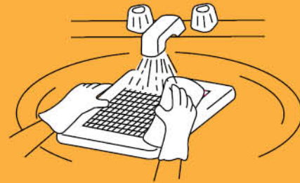
2. Wash and clean louver.
