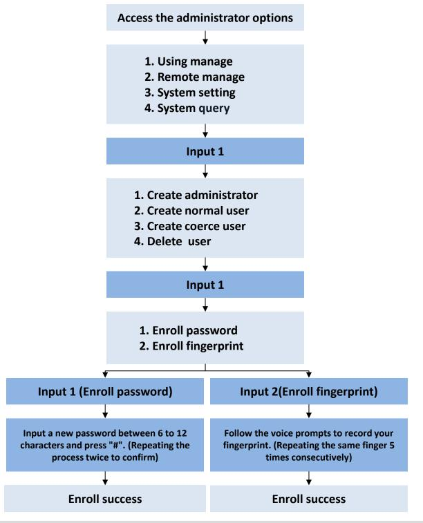
Note: After successful fingerprint enrollment, the system will automatically proceed to the next number. If you wish to stop, press "\*" to exit.
