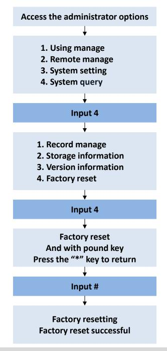
Note: You can also restore the factory settings by holding down the "Unlock" and "Lock" on the rear panel simultaneously;
