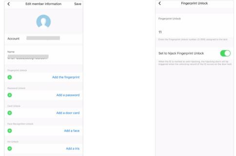
Attention: When using a hijack alarm user to unlock the door, the lock will open normally without sounding an alarm. However, an alarm message will be pushed to the App. But if the door lock is not connected to the network when the door is unlocked, the alarm information will not be uploaded to the cloud.
